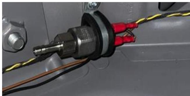
Plug the two red plugs into the pressure switch and connect this to boost pressure.
