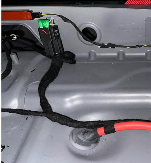
Pass the cable through the tunnel on the bulkhead, route it towards the fuel pump and connect the cable to the HPerformance fuel pump.
