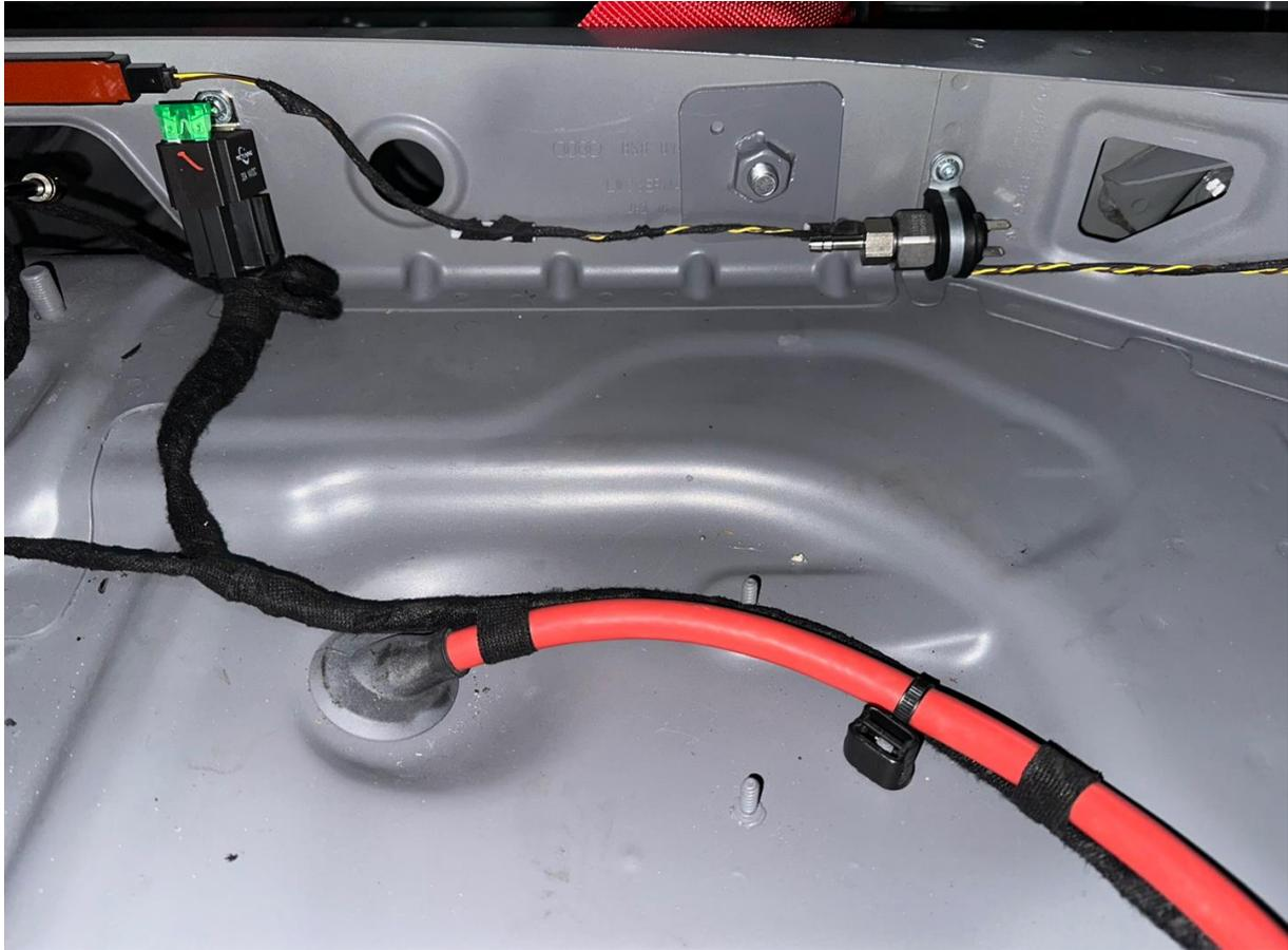
Fasten the relay and the pressure switch to the fastening points as shown in the picture.
